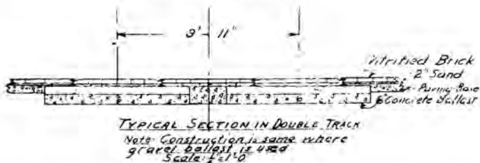
Cross-section of standard double-track grading as used by Portsmouth Street Railroad & Light Co.
