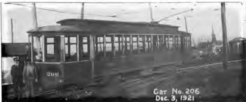
PSRR&LC car No. 206, shown December 1921, was constructed by St. Louis Car Co. in 1904. Similar to the 100-series Brill cars, the 206 likewise was improved in 1917. CITY OF PORTSMOUTH, 1921 COMPANY AUDIT
