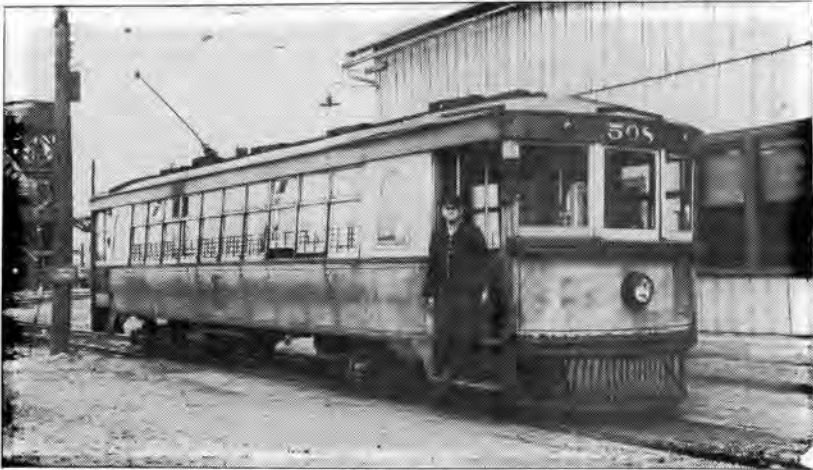
Portsmouth Public Service Co. No. 508, built by Cincinnati Car Co. in 1925, shown here beside Second Street car barn. was one of three (506-508) used both for city and interurban service. THOMAS D. DRESSLER COLLECTION
